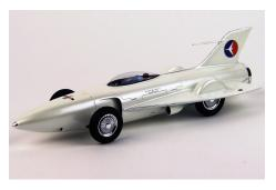
turbine-powered car tested in the US. It was entirely impractical, with a bubble top canopy over a single seat cockpit, a bullet shaped fuselage made entirely of fiberglass, with short wings, and a vertical tail fin. It had a 370 hp Whirlfire Turbo Power gas turbine engine, which has two speeds, and expels jet exhaust at some 1,250° F (677°C). The car weighed only 2,500 lb, and sat on a 100" wheelbase. This resin replica (preproduction sample photos) is expected in March.
